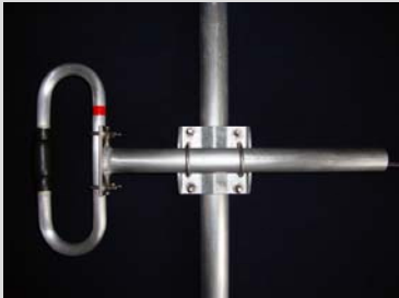
1/4 - wave spacing (5.95 - 8.5 dBd gain) (Omnidirectional - Offset pattern)
